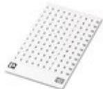
Marker card, white, labeled, horizontal: consecutive numbers 1 ... 10, 11 ... 20, etc. up to 91 ... (99)100, mounting type: adhesive, for terminal block width: 5.08 mm, lettering field size: 5.08 x 3.8 mm
